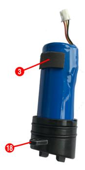
e. Hold the Control Pod internal wiring loom [12] firmly with your finger and thumb and connect the battery cable to the wiring loom ensuring that the white connector of the wiring loom from the Control Pod is flush with the entrance of the battery compartment while doing so.
